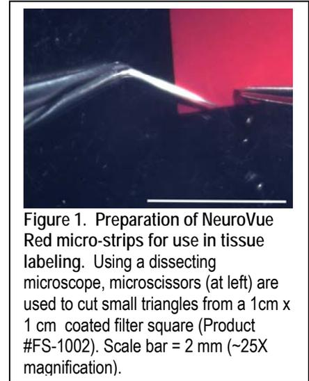
Figure 1. Preparation of NeuroVue Red micro-strips for use in tissue labeling. Using a dissecting microscope, microscissors (at left) are used to cut small triangles from a 1 cm x 1 cm coated filter square (Product #FS-1002). Scale bar = 2 mm (~25X magnification).
